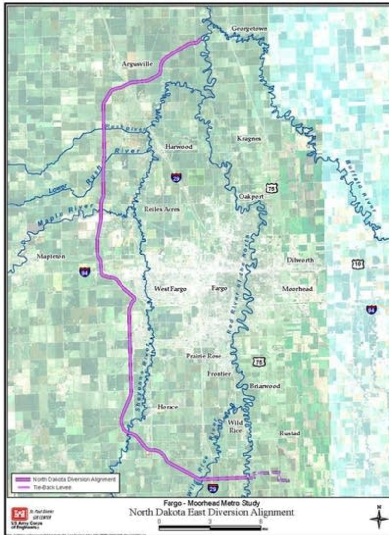
Figure 16 - North Dakota East diversion alignment
