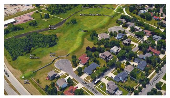
An engineer's rendering shows the location of a levee and floodwall to be built in the Rose Creek area. The city plans to use eminent domain on a property at 4122 17th St. S. It's not pictured but would be to the right of the word "levee." Source: city of Fargo.
