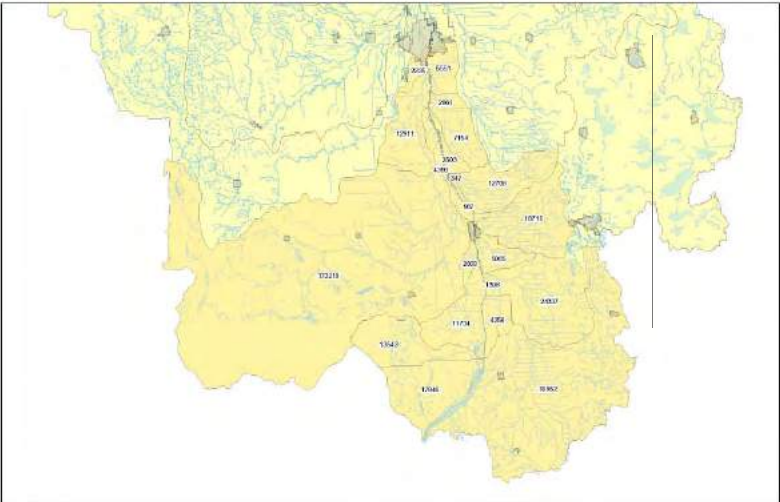
Figure 5. High estimate of potential storage for the various watersheds upstream of the communities of Fargo, North Dakota and Moorhead, Minnesota.
