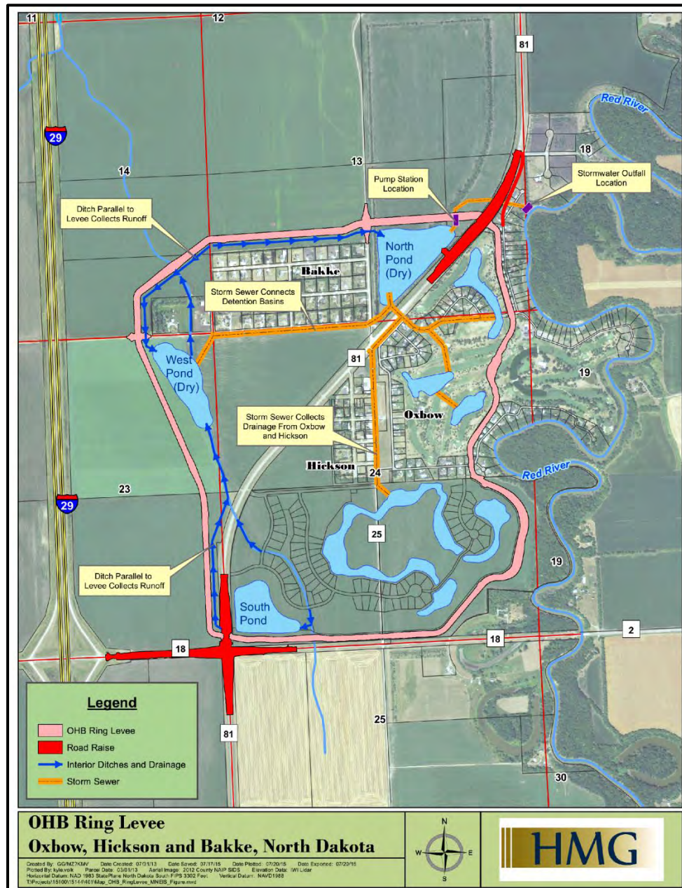
ES Figure 3 Oxbow/Hickson/Bakke Ring Levee Design
