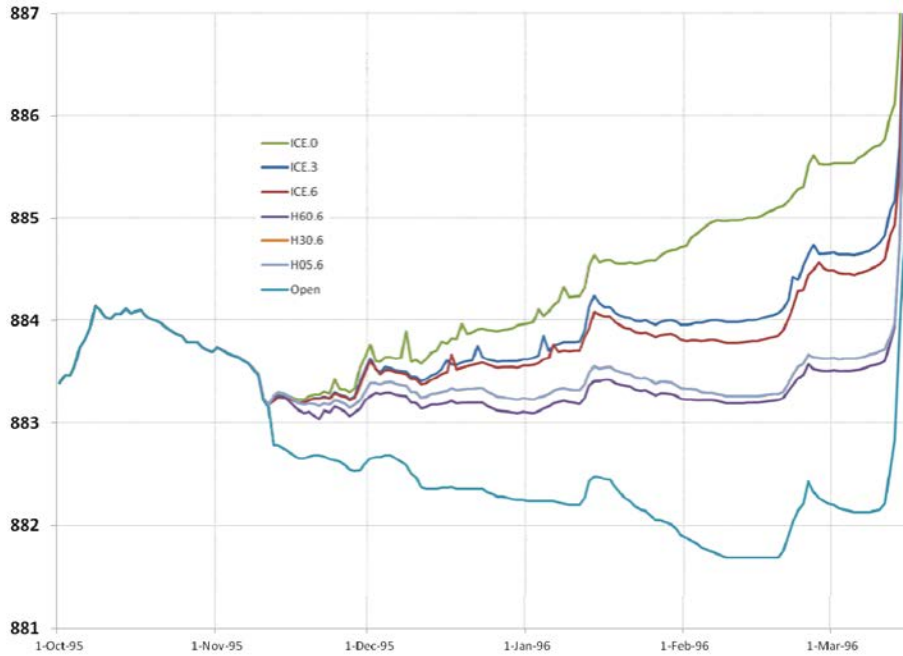
4647 Graph 3.3: Upstream Water Levels for Water Year 1996 for Different Scenarios and for Open Water
