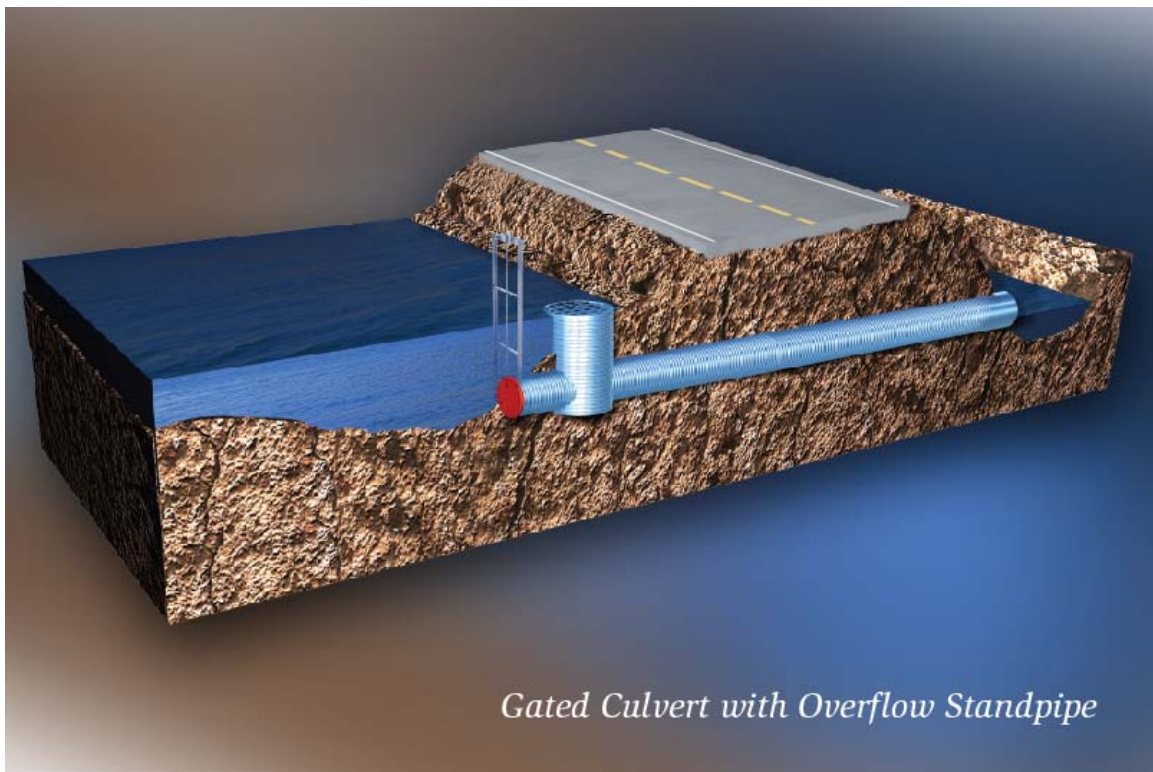
Figure 6. Water retention in Waffle storage section using gated culvert and overflow standpipe.
