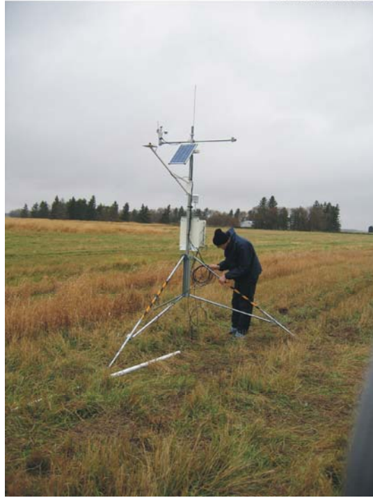
Figure 50. Photograph of meteorological station being installed.
